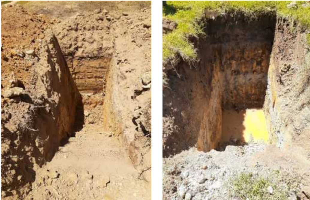
Figure 4-5: Elastic silt at TP4 and TP5 (note ground water in TP5)
